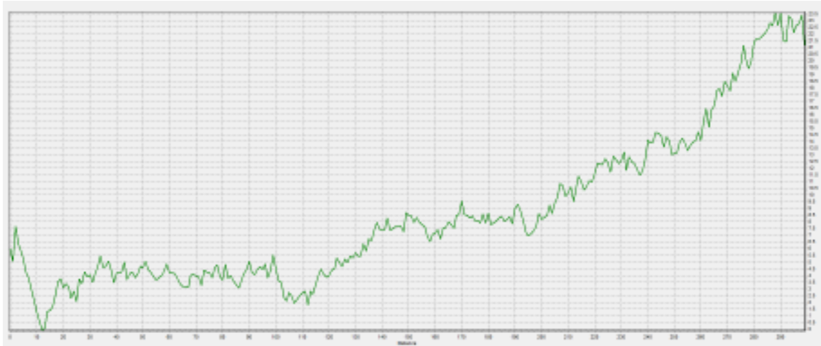
Figure 4 – The Damage Index shows how the non-linear response changes over the scan.
